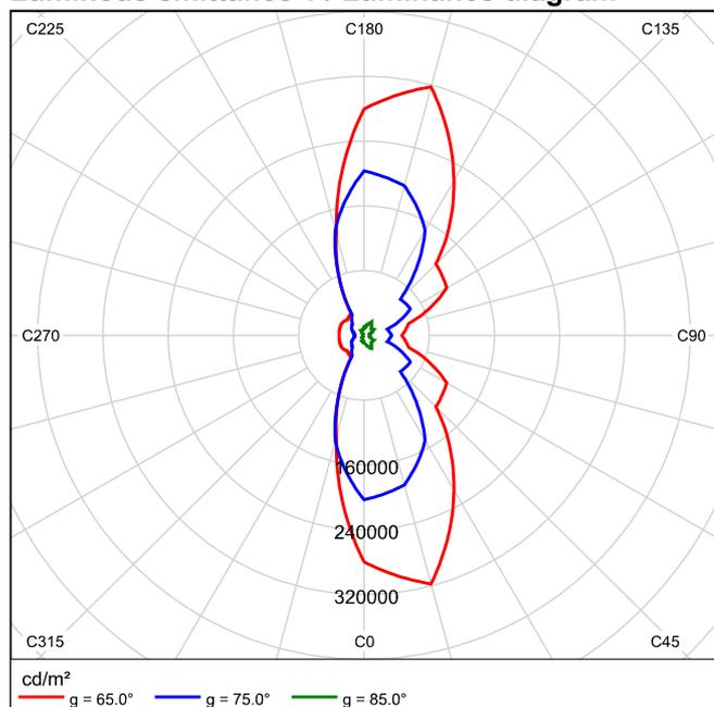
It is not possible to generate a UGR diagram, as the light distribution is asymmetrical.
